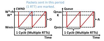
Fig. 16. AIMD Sawtooth illustration.
