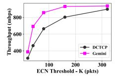
Fig. 8. Aggregate throughput of inter-DC flows that bottlenecked at a DCN link. GEMINI is less buffer-hungry (requires 0-76% smaller K) than DCTCP when achieving similar throughput.
