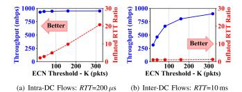
Fig. 5. Conflicting ECN requirements in DCTCP. The right y-axis shows latency by the inflated RTT ratio—the queueing-inflated RTT normalized by the base RTT (w/o queueing).
