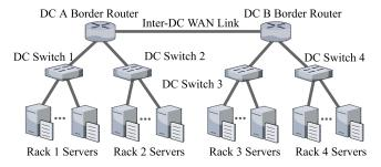
Fig. 3. Cross-datacenter network testbed.
