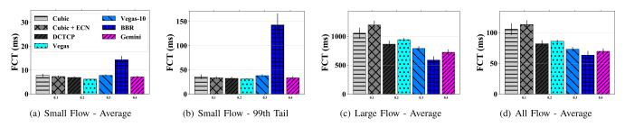
Fig. 15. [Small-scale 10 Gbps testbed] FCT results under traffic pattern 2: mixed inter-DC and intra-DC traffic, highly congested both in WAN and DCN. Small flow: Size  $< 100 \, \text{KB}$ . Large flow: Size  $> 10 \, \text{MB}$ .
