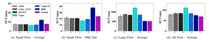
Fig. 13. [Small-scale 10 Gbps testbed] FCT results under traffic pattern 1: Inter-DC traffic, highly congested in WAN. Small flow: Size < 100 KB. Large flow: Size > 10 MB.
